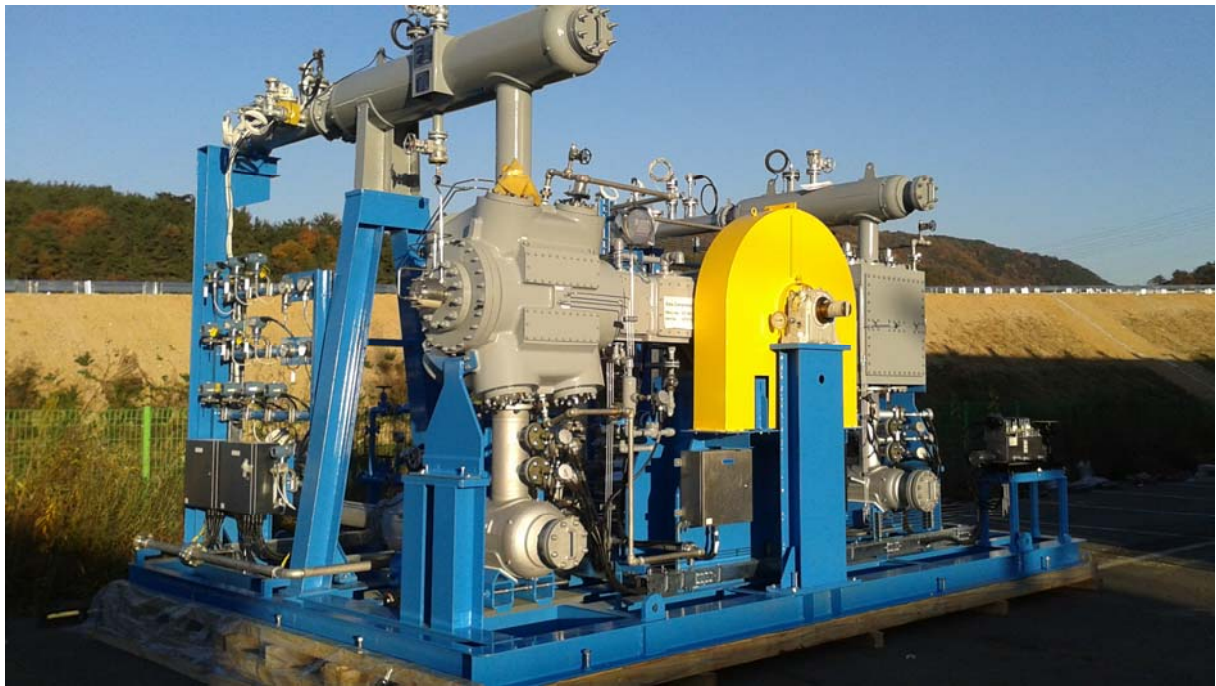
Product name API Reciprocating Gas compressor (6sets) Customer NEA(Neuman & Esser) / Fu-tai Engineering Specification Full skid mounted 2stg
