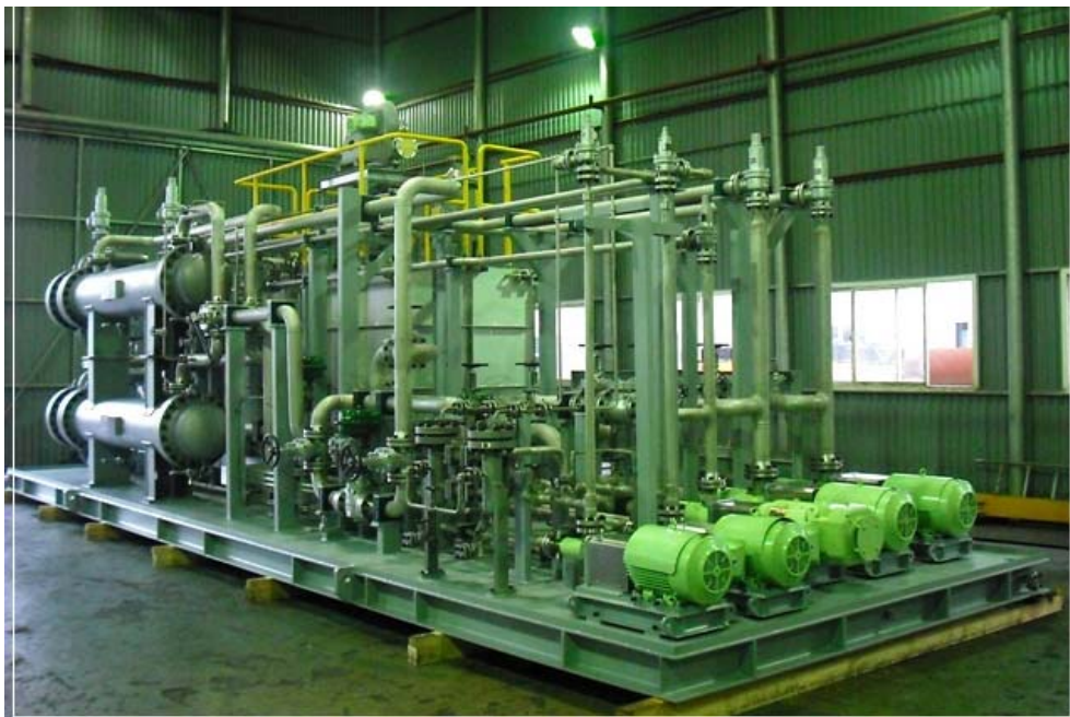
Product name Lube & Control oil console for 15MW Steam turbine Customer Mitsui Engineering & Shipbuilding Co., Ltd. Specification SA312-316 / 750LPM / ASME "U" stamp & API, 3.5m(W)x12m(L)x4.2m(H)x25ton
