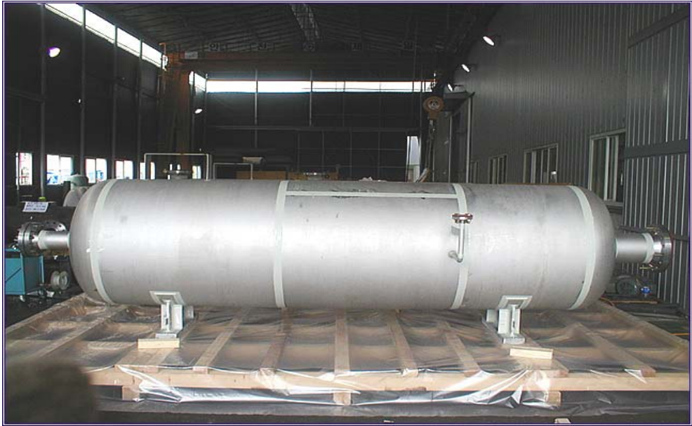
Product name Surge Drum Customer KOBELCO, TECHNIP / USA Specification SA240-316 / 12t / 22.9kg/cm 2 / ASME "U" stamp / NB
