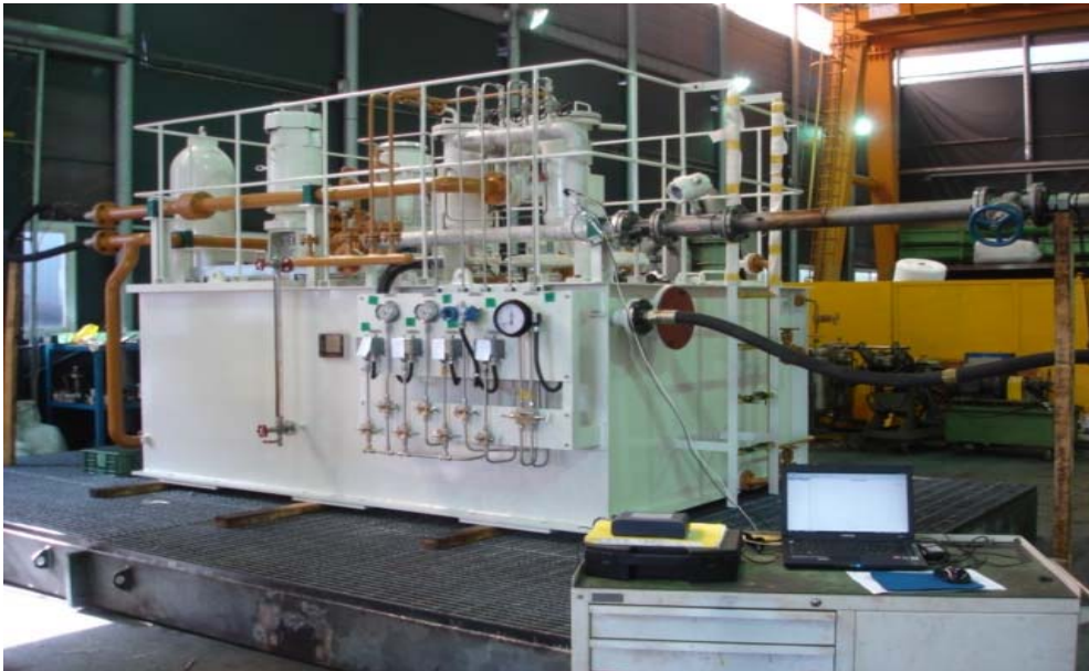
Product name Lube oil console for 60MW Steam turbine Customer FUJI Specification SA106-B / 40m3/hr /MOP,EOP
